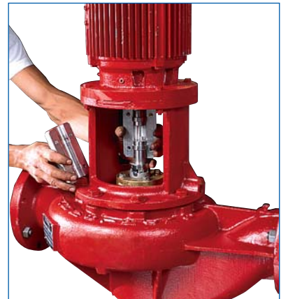
2) Remove the coupling bolts. The coupling halves (with drive and annular positioning keys) are taken from motor and pump shafts. Loosen set screws on seal rotating element and slide from pump shaft. (For inside seal see step (3))
