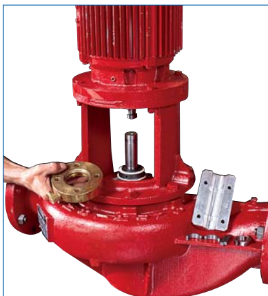
3) Disconnect seal flush line and remove gland plate bolts. The gland plate and seal seat may then be taken out between the space in the shafts. With inside seal the complete seal is removed following the gland plate.
