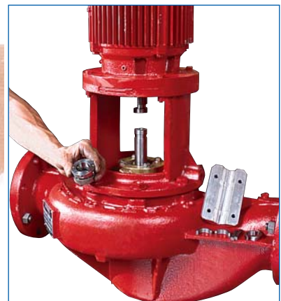
4) New seal may now be installed. Reverse the procedure: Install new seal, replace gland plate, replace coupling and restart pump. Rigid coupling retains factory alignment.
